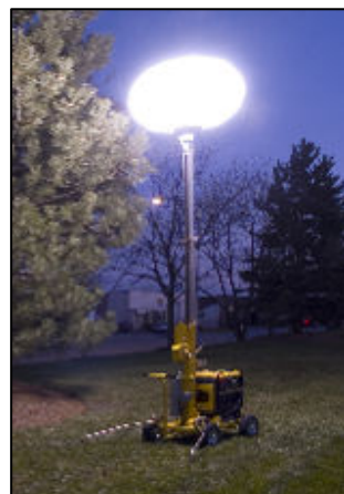
Inverter Generator and Light Tower
